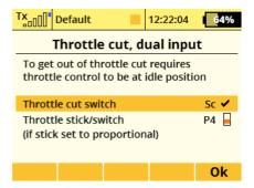
Select the switch you want to use, it must be on when throttle cut is to be active.
