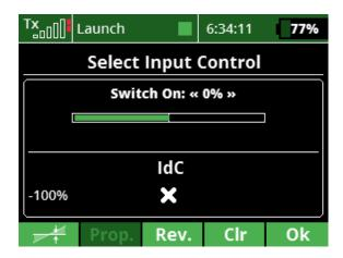
Please note that the Throttle-Cut Switch needs to be reversed in order to properly work.
