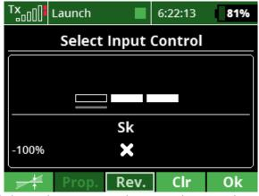
In order to attain the control to be ON when not in Flight Mode 1, I reverse this particular control.
