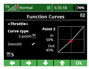
I do this in order to have the exact feeling on all the throttle range. What the Throttle Idle offset really does, it reduces the overall range of the throttle, so by adjusting the curve I'm able to have a seamless experience on the throttle range.
