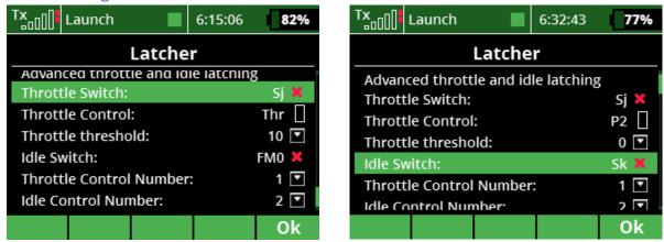
The Configuration screen of the Latcher has six parameters:
