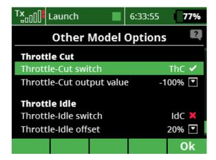
For this, you need to add the following user controls, 1 and 2 (or ThC and IdC). For Throttle-Cut Switch:
